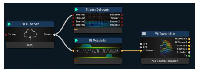
When sending data to the Tx port of a transmitter, it is important to keep the target time some 100ms in the future to allow for network and processing delays.
