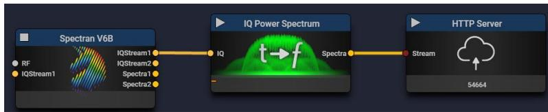
Including a demodulation block allows fine grained control of the spectrum range and sample rate down to the sub hertz frequencies.
