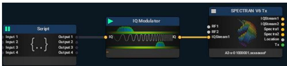
The modulator block is used for up-conversion, data rate adaptation and frequency shift.
